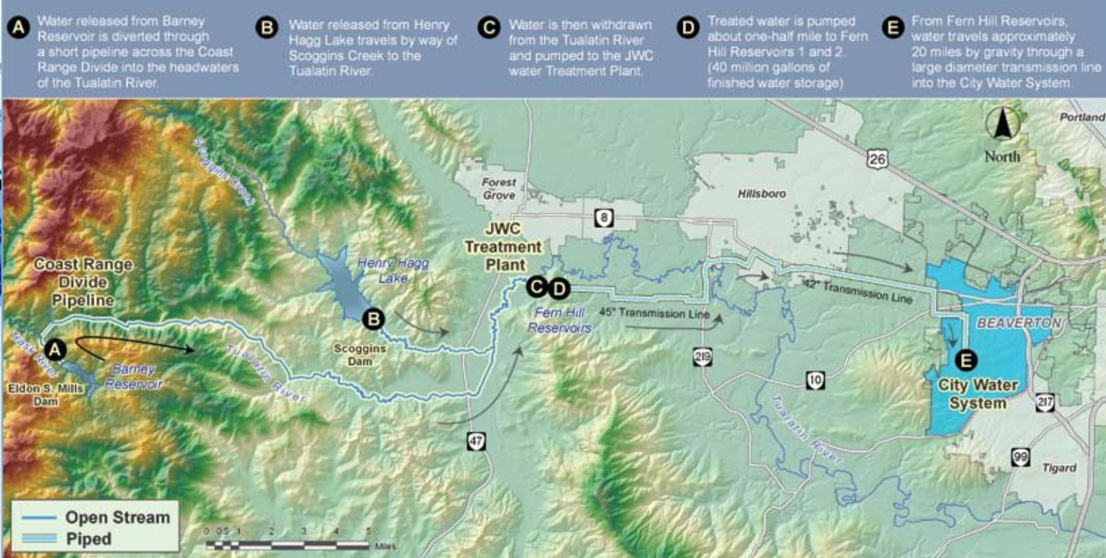
**A** Water released from Barney Reservoir is diverted through a short pipeline across the Coast Range Divide into the headwaters of the Tualatin River.
