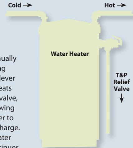
Manually lifting the lever unseats the valve, allowing water to discharge. If water continues to leak from the T & P Valve after closing, the valve may need to be replaced. A drain line must be installed to avoid water damage and scalding injury when the valve operates. The T & P Valve should be removed periodically and visually inspected for corrosion deposits and to ensure it has not been improperly altered or repaired. The above work can best be done by a licensed plumber.
